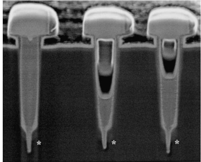
FIG. 4. Cross-sectional image of 2.4  $\mu\text{m}$  deep 0.4  $\mu\text{m}$   $\times$  0.4  $\mu\text{m}$  HAR vias, gradually filled with tungsten by the 0.1  $\mu\text{m}$   $\times$  0.1  $\mu\text{m}$  deposition box. The small tip at the bottom of the vias was caused by precursor gas depletion and milling by relatively high ion beam current during deposition.
