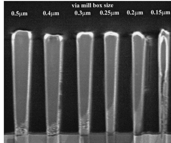
FIG. 6. Cross-sectional image of the series of  $5\ \mu\text{m}$  deep vias milled by FIB in  $\text{SiO}_2$  dielectric substrate and filled void free with tungsten by deposition boxes measured 1/4 of the via size for vias with aspect ratio in range from 10:1 ( $0.5\ \mu\text{m} \times 0.5\ \mu\text{m}$ ) to 25:1 ( $0.2\ \mu\text{m} \times 0.2\ \mu\text{m}$ ), based on via mill box size.
