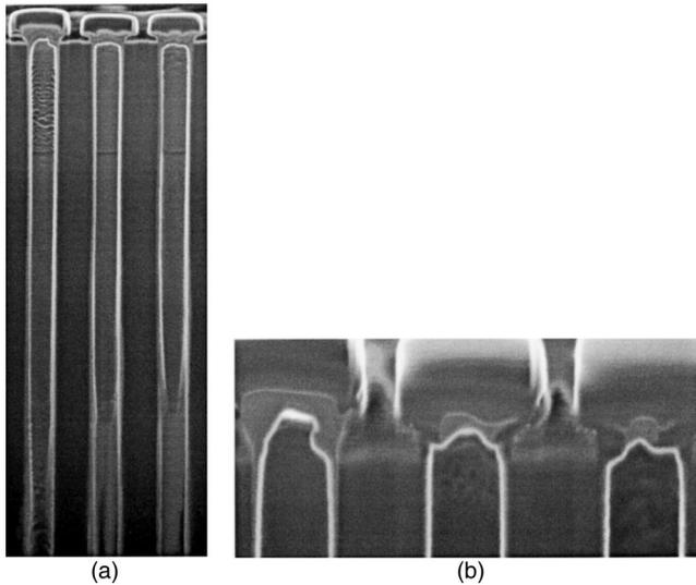
FIG. 5. Cross-sectional image of  $0.5\ \mu\text{m} \times 0.5\ \mu\text{m}$  UHAR vias with  $>40:1$  aspect ratio, showing bottom-up fill by  $0.15\ \mu\text{m} \times 0.15\ \mu\text{m}$  deposition at the beginning of the deposition (a) and interruption of the filling process due to closing of via aperture (b).
