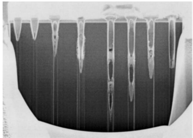
FIG. 1. Cross-sectional image of series of 0.5  $\mu\text{m}$  × 0.5  $\mu\text{m}$  vias with depth ranging from  $\sim$ 3 to  $\sim$ 10  $\mu\text{m}$ , filled with tungsten by the 0.35  $\mu\text{m}$  × 0.35  $\mu\text{m}$  deposition box, shows formation of large deposition voids in HAR vias.
