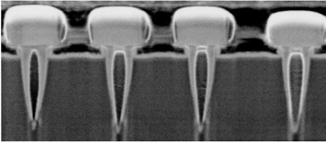
FIG. 3. Cross-sectional image of 1.5  $\mu\text{m}$  deep 0.5  $\mu\text{m}$   $\times$  0.5  $\mu\text{m}$  LAR vias, filled with tungsten by the 0.6  $\mu\text{m}$   $\times$  0.6  $\mu\text{m}$  deposition box. Large voids within the deposited material are the indication of incomplete via fill.
