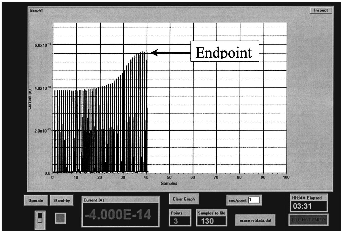
FIG. 2. Main screen of experimental TESTPOINT data plotting application with the typical shape of the plot observed on the sample absorbed current monitoring setup at the endpoint of the via fill deposition. X axis represents consequent current sample number in arbitrary units.
